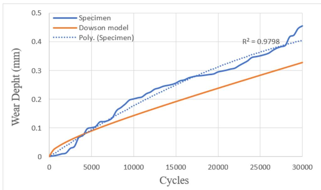
Fig. 5. Validation of test with Dowson model
