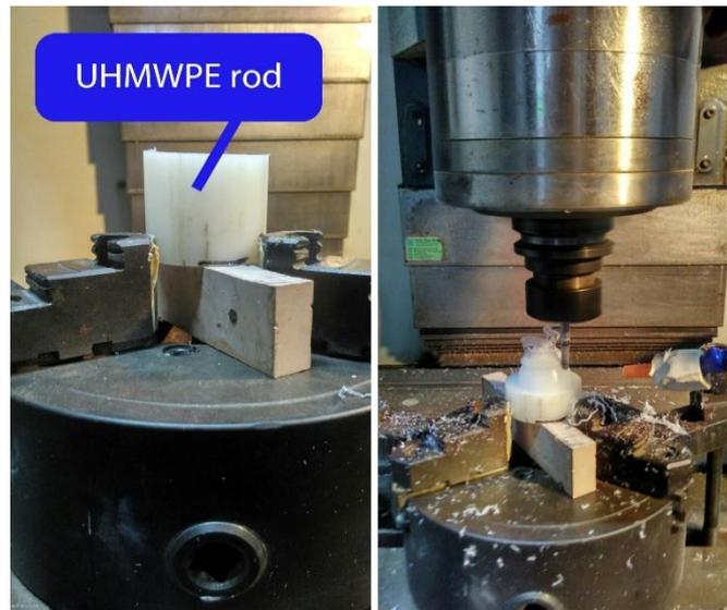
Fig. 1. Experimental set up for the milling of UHMWPE acetabular liner
