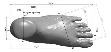
Fig. 2. Foot scan measurement (unit length in mm)
