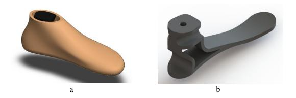
Fig. 3. The design of (a) skin part, and (b) supporting core of ankle foot
