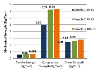
Fig. 3. Mechanical Properties of Sand Moulds in Wet Conditions
