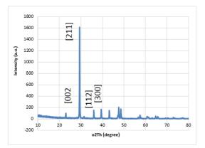
Fig. 2. Phase Identification of Eggshell Nanopowder without Sintering at 1100°C
