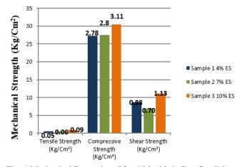
Fig. 4. Mechanical Properties of Sand Moulds in Dry Conditions
