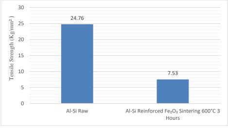
Fig 1. Comparison of the tensile strength of Al-Si alloy
