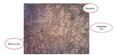
Fig 3. The microstructure of Al-Si raw material
