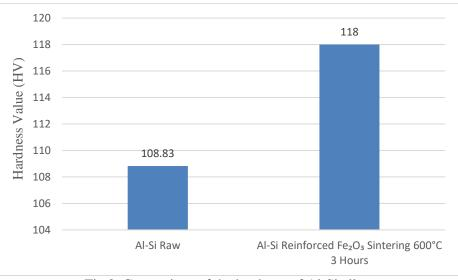
Fig 2. Comparison of the hardness of Al-Si alloy
