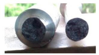
Fig 6. Morphology of Al-Si alloy reinforced by Fe<sub>2</sub>O<sub>3</sub>
