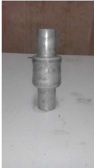
Figure 5. The hydroformed stepped tube with the proposed die and mechanism
