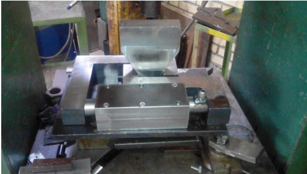
Figure 3. The die set mounted on the test machine
