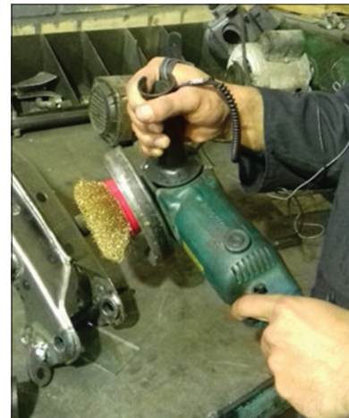
Figure 2: The heavy duty right angle sander to finish or polish metal
