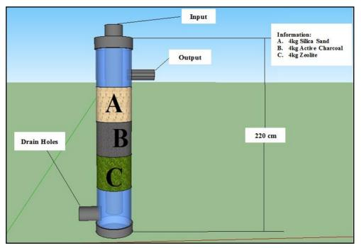
Figure 1. Design of Filter Tube Media (Source: Primary Data, 2017)
