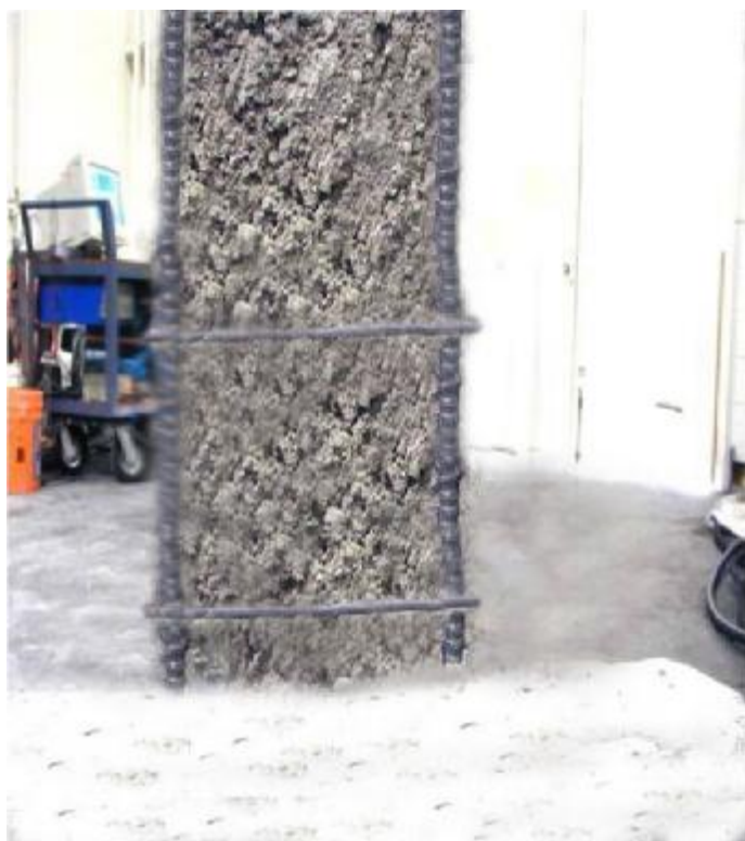
Figure (9) : Removing of cracked shell of specimen A2
