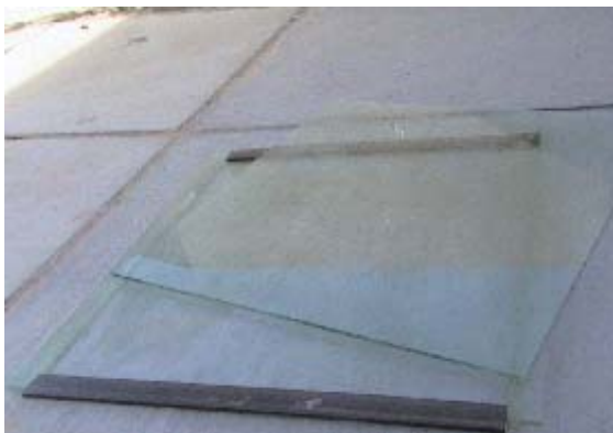
Figure (6-a) Glass casting mold
