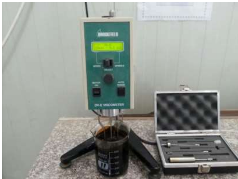
Figure (1): Brookfield digital viscometer model DV-E in the Lab.
