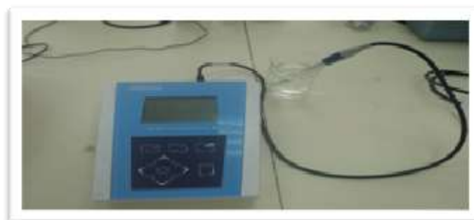
Figure (2): Conductivity meter
