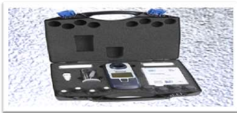
Figure (3): Turbidity meter
