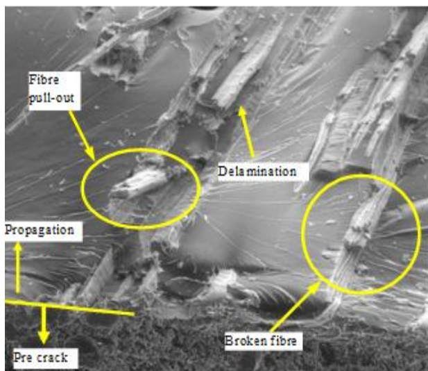
Figure 9: Fracture surface of ut-KFRE composites in Y-direction.
