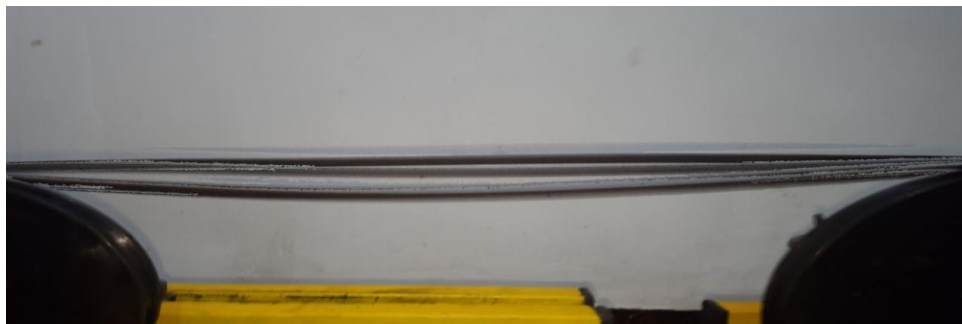
Figure 4: stroboscope camera picture shows belt resonance.
