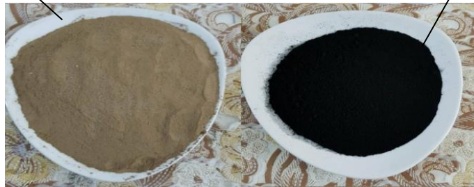
Figure 5. conocarpus-without chemically treated and carbonized conocarpus, materials used as adsorbents in the present study.
