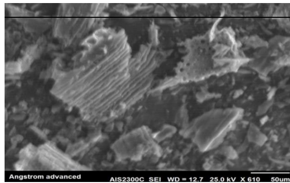
Figure 3. SEM micrograph of activated carbon.
