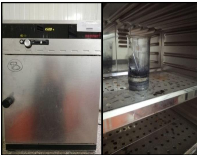
Figure 1. photographic picture of the apparatus used for coating sand with graphene oxide.
