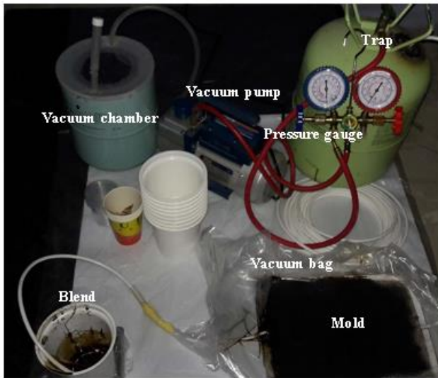
Figure 2. Vacuum infusion technique
