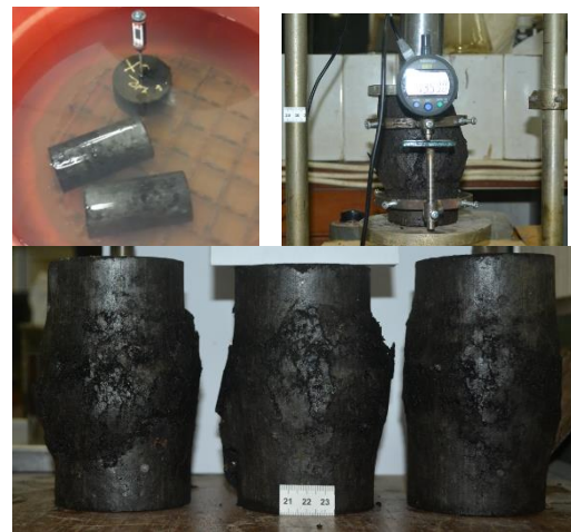
Figure 6. (a) Specimen immersion; (b) specimen UCS test; (c) specimen after UCS test
