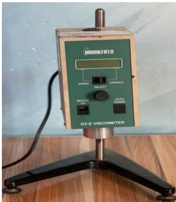
Figure 1. DV-E Viscometer used for viscosity measurements.
