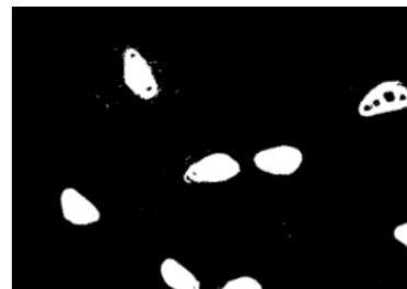
Figure 5. Segmentation stages, create a mask using Otsu Thresholding
