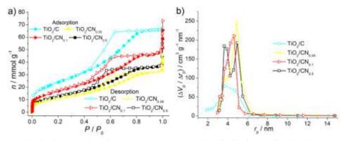
Fig. 4. Nitrogen adsorption isotherms (a) and pore size distribution (b) for  $TiO_2/C$  and  $TiO_2/CN$  samples.
