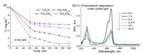
Fig. 7. Photocatalytic decomposition of MB in the presence of undoped and N-doped samples (a) and absorption spectra of MB on  $TiO_2/CN_{0.05}$  (b).
