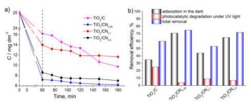
Fig. 6. Photocatalytic decomposition (a) and removal efficiency (b) of MB in the presence of  $TiO_2/CN$  composites.
