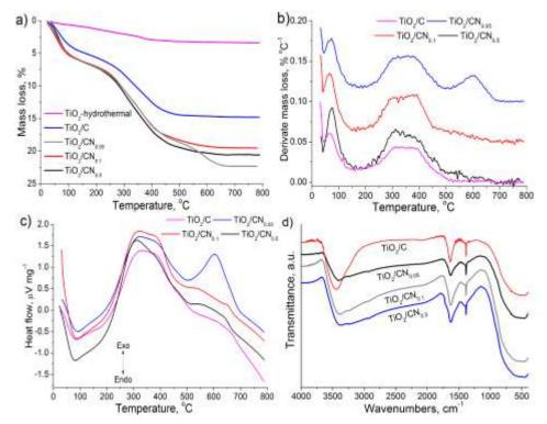
Fig. 2. TGA (a), DTG (b) and DTA (c) curves, and FTIR spectra (d) of TiO<sub>2</sub>/C and TiO<sub>2</sub>/CN composites.
