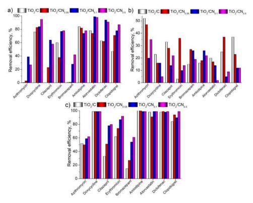
Fig. 8. Removal of pharmaceuticals from a multi-component solution by  $TiO_2/C$  and  $TiO_2/CN$  composites: a) adsorption in the dark, b) under UV irradiation and c) total removal.
