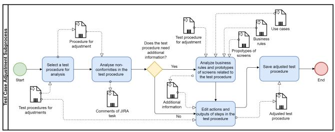
Figure 8. Subprocess to Adjust Test Procedure.
