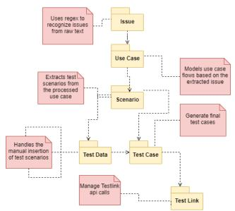
Figure 2. Package Diagram of developed UC2Proc.
