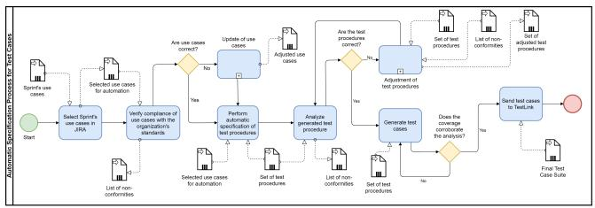
Figure 7. Process to Semi-Automatic Specification of Test Procedures.
