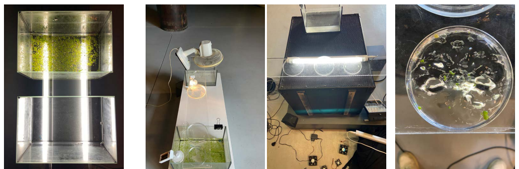
Figures 12 to 15: Vibration experiments . Fans, subwoofer and Lemna gibba . Water movement, disturbance and vibration at different frequencies.
