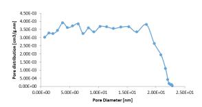
Figure 4. Distribution of pore diameter for golden snail after decomposition at 900 oC.
