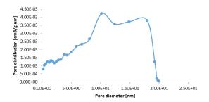
Figure 5. Distribution of pore diameter for lion snail after decomposition at 900 oC.
