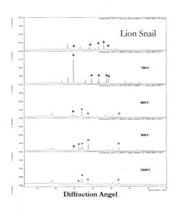
Figure 2. XRD powder patterns of decomposition of lion snail shell at various temperatures.
