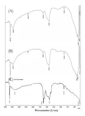
Figure 3. FTIR spectrum of calcium oxide standard (C) and decomposed from golden snail (B) and lion snail shells (A).
