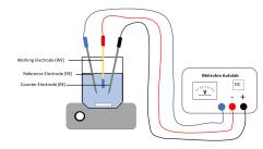
Figure 2. Electrochemical Cell
