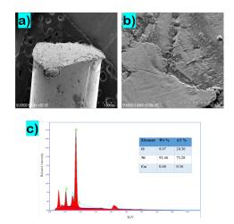
**Figure 3.** Morphology Scanning Electron Magnetic (SEM) of Material Ni/EC Surface with Magnification 5 Times (a), 5000 Times (b) and Result of Energy Dispersive X-Ray (EDX) from SEM Data Surface Electrode Ni/EC (c)
