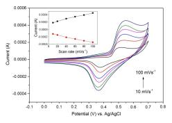
**Figure 8.** Cyclic Voltammogram of Various Scan Rate (10-100 mVs<sup>-1</sup>) in 0.001 M Glucose
