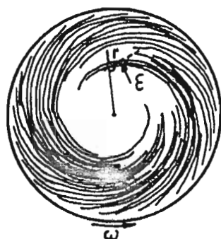
Fig. 10. Scheme of the rotating disk with spiral vortices
