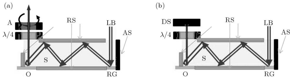
Fig. 8. Polarization phase shift sensor heads: (a) with rotational analyzer and (b) with dynamic wavefront sensor (Patorski and Kujawinska, 1993); RS – reflective surface, LB – laser beam, AS – absorbing surface, RG – reference grating, O – Object, S – Spacer,  $\lambda/4$  – quarter waveplate, A – analyzer, DS – dynamic wavefront sensor (Millerd *et al.*, 2005)
