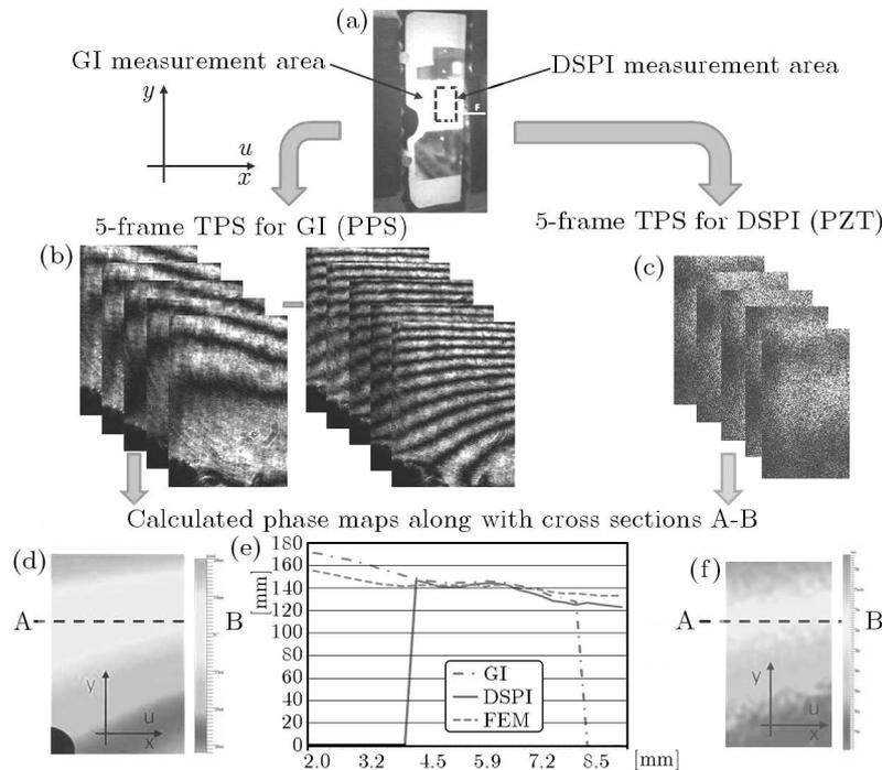
Fig. 10. Results of measurements: (a) specimen, (b) set of phase shifted interference fringes in two subsequent object states for GI mode, (c) set of phase shifted correlation fringes for DSPI mode, displacement maps (d) for GI, (f) for DSPI and (e) cross sections showing absolute values for both modes and FEM model
