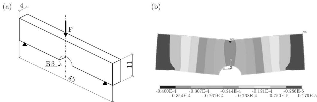
Fig. 9. Specimen used for measurements (a) along with its FEM model (b)
