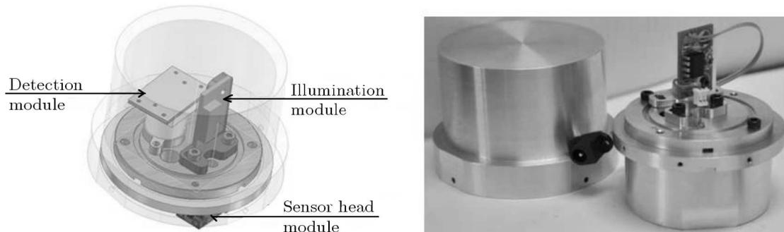
Fig. 1. Basic scheme and photo of the coherent sensor utilizing the hybrid method
