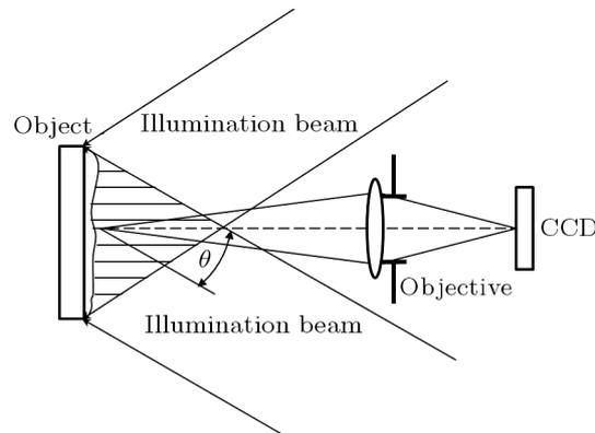
Fig. 4. Basic ESPI system for in-plane displacement measurement
