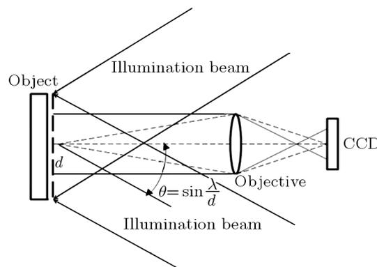
Fig. 2. Principles of grating interferometry for in-plane displacement measurement
