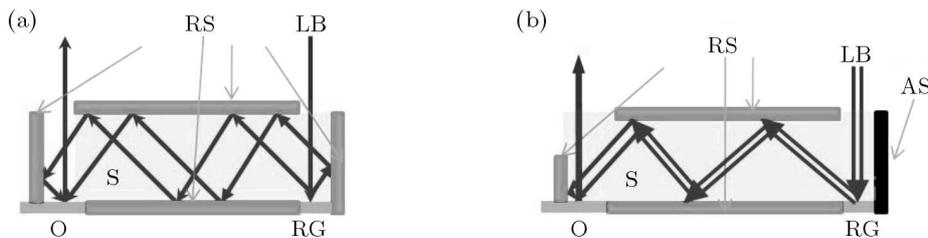
Fig. 5. Proposed sensor heads (a) with equal number of reflections of both interfering beams – (A) and (b) with different number of reflections of each interfering beams – (B); RS – reflective surface, LB – laser beam, AS – absorbing surface, RG – reference grating, O – Object, S – Spacer
