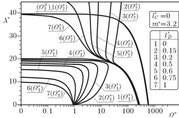
Fig. 12. Curves on the plane: loading parameter – parameter of natural vibration frequency of column **B**
