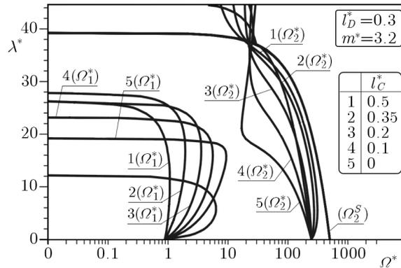
Fig. 13. Curves on the plane: loading parameter – parameter of natural vibration frequency of columns for various parameters  $l_C^*$
