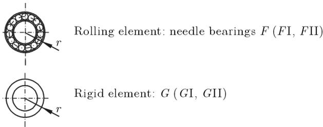
Fig. 3. Elements used in the rotary elements of the forcing head
