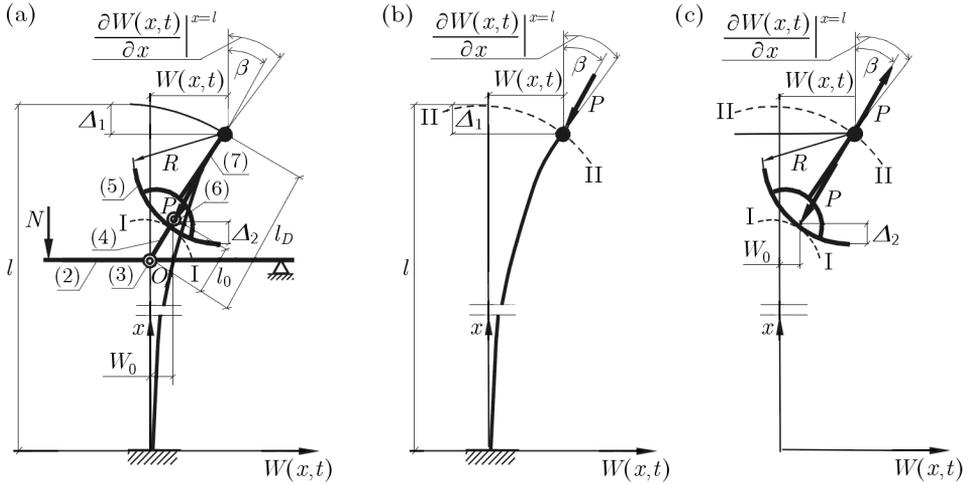
Fig. 5. Deflected form of column **B** (see Fig. 2b), geometry and externalisation of internal forces
