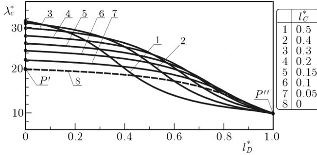
Fig. 10. Change of the critical parameter of load  $\lambda_c^*$  against the parameter  $l_D^*$  for various values of  $l_C^*$
