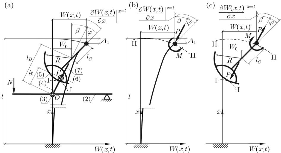
Fig. 4. Deflected form of column type A (see Fig. 2a), geometry and externalisation of internal forces
