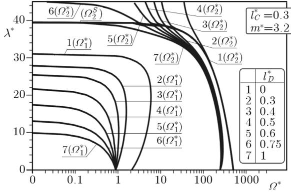
Fig. 11. Curves on the plane: loading parameter – parameter of natural vibration frequency of column **A**
