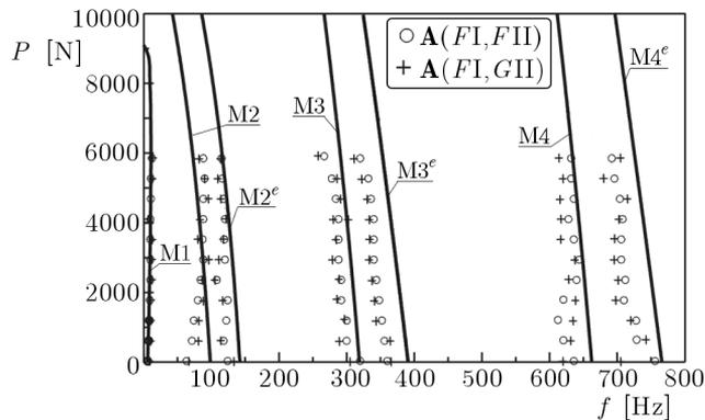
Fig. 8. Curves in the plane: load – natural frequency for columns **A**
