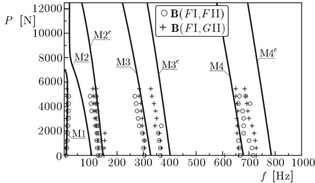
Fig. 9. Curves in the plane: load – natural frequency for columns **B**
