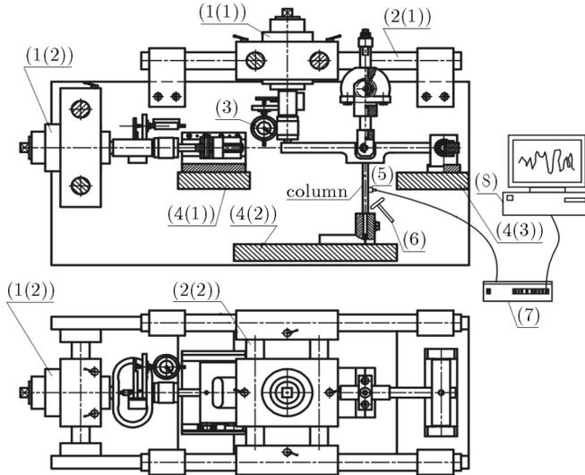
Fig. 7. Test stand for experimental research of the considered columns
