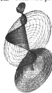
Fig. 9. Modal shapes and natural frequencies of the rotor for forward and backward precession
