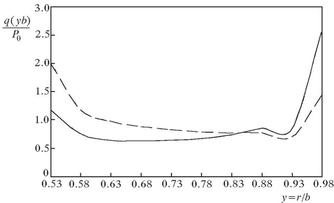
Fig. 2. Contact stresses  $q(yb)/P_0$ ,  $\lambda = a/b = 0.5$
