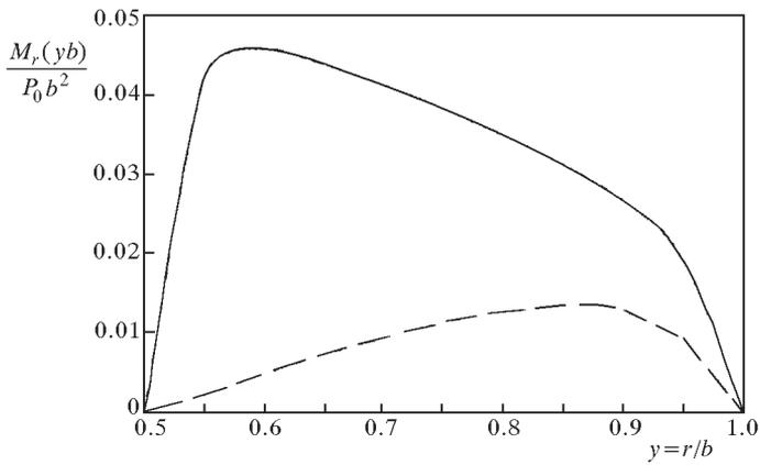
Fig. 4. Bending moment  $M_r(yb)/(P_0 b^2)$ ,  $\lambda = a/b = 0.5$
