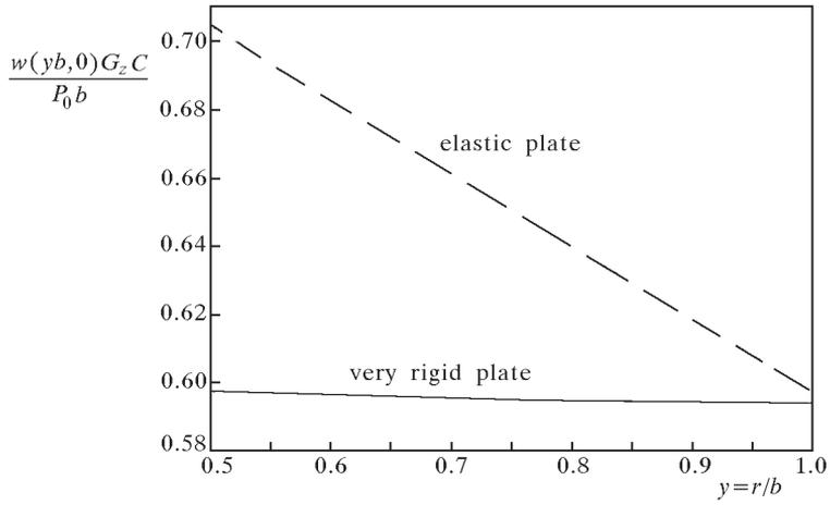
Fig. 3. Transverse deflection of the plate,  $\lambda = a/b = 0.5$
