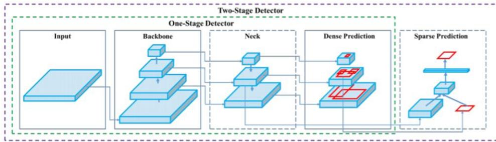
Fig. 6. YOLOv4 model architecture [16]
