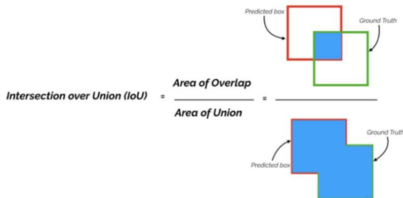
Fig. 7. Calculation of IoU
