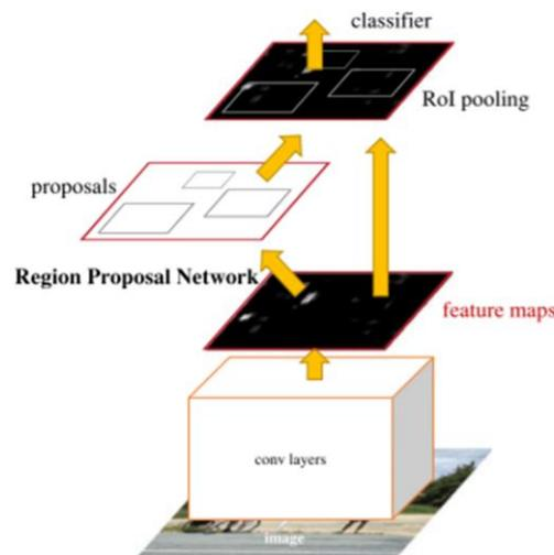
Fig. 4. Faster R-CNN model architecture [11]
