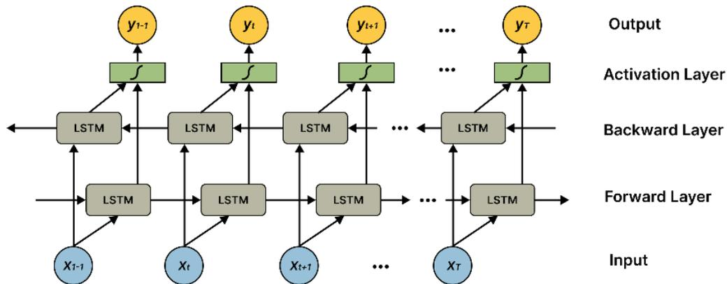
Fig. 6. Bi-LSTM Architecture
