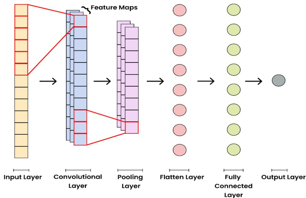
Fig. 3. 1D-CNN architecture
