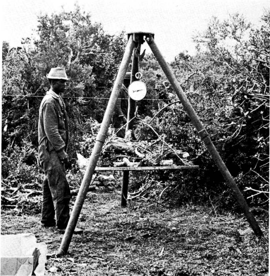
Fig. 4. The tripod and spring balance used for determining the sample mass. Note the dense vegetation (outside the elephant camp).
