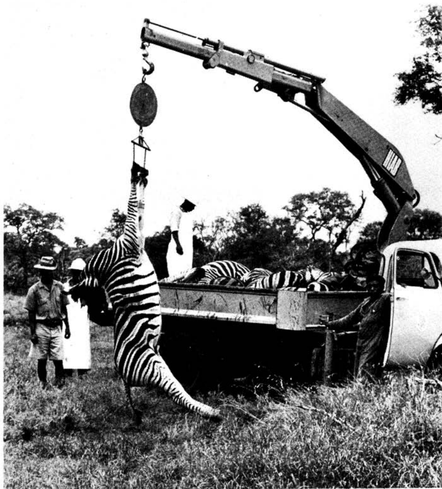
Fig. 2. The "Hiab" hydraulic hoist and the attached heavy duty "Salter" spring scale (0-510 kg) used for measuring body mass.
