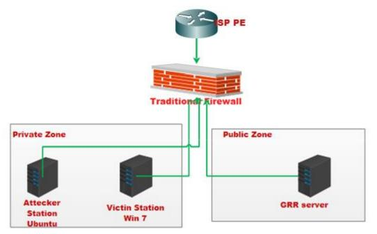
Figure 2. Experiment Setup Topology
