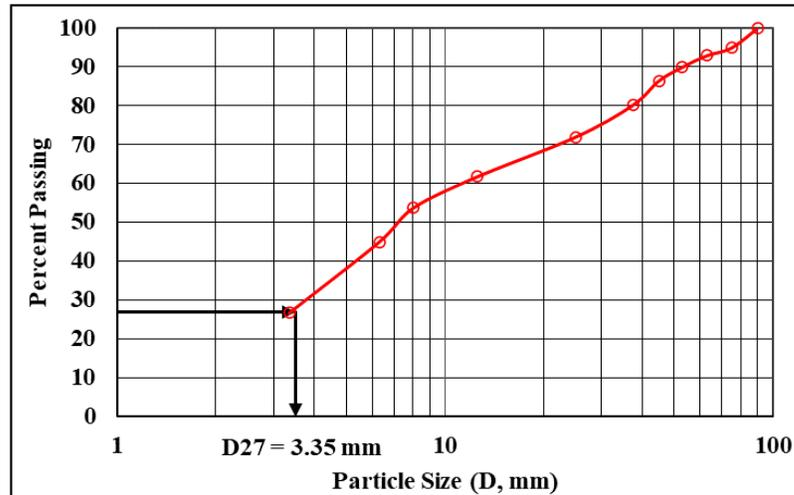
Figure 5. PSD of Runoff Mine Stockpile Coal at the MCM. D27 is the size of the sieve from which 27% of the coal is passing.
