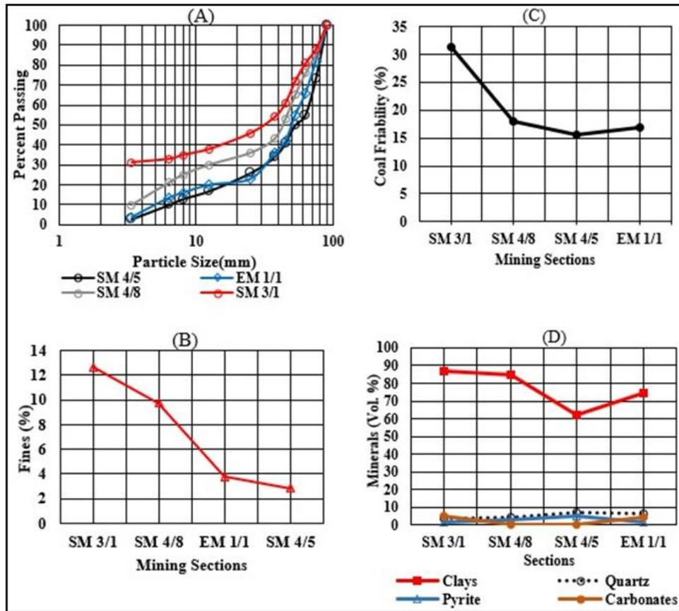
Figure 4. Coal samples from the MCM: (A) Particle Size Distribution curve, (B) Fines (%), (C) Friability (%), and (D) Minerals present in four sections (Vol.%) (Saubi et al., 2022).
