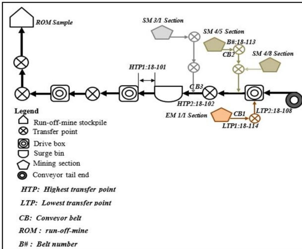
Figure 2. Location of sample points at Morupule Coal Mine.
