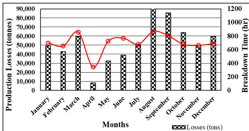
Figure 10. Relation between Production Losses and Conveyor Breakdowns at the MCM.
