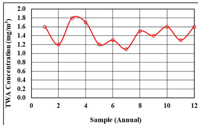
Figure 13. Underground coal dust concentration in MCM.
