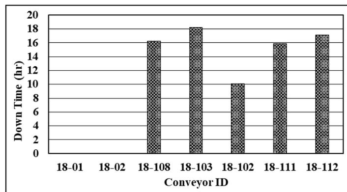
Figure 8. Blockages for Individual Conveyors at the MCM.
