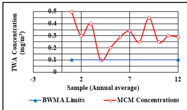
Figure 11. Surface Coal Dust Concentration in MCM.
