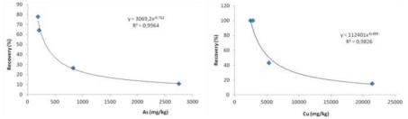
Fig. 3. Relationship between recovery of elements (As, Cu) during bacterial leaching and concentration of elements in waste rock.
