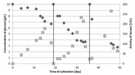
Fig. 3. Repeated-batch cultivation of *C. subvermispora* in cultivation medium with 10 g/L of glucose and 1.5 g/L of casein hydrolysate at 30 °C and pH 5.0;  $\bullet$  - concentration of glucose and  $\blacksquare$  – activity of laccase.
