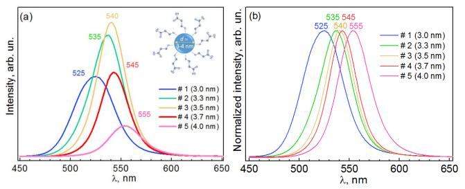
**Fig. 1.** Photoluminescence spectra of the CdTe QDs used in this work (measured in parental solutions). Absolute PL intensity is in (a) and (b) shows spectra with normalized intensity for better visibility of different peaks position for different samples (indicated on both figures). The inset to (a) schematically shows the QD stabilized by the ligand (TGA). Hereinafter: #1-5 are numbers of QD experimental solutions.
