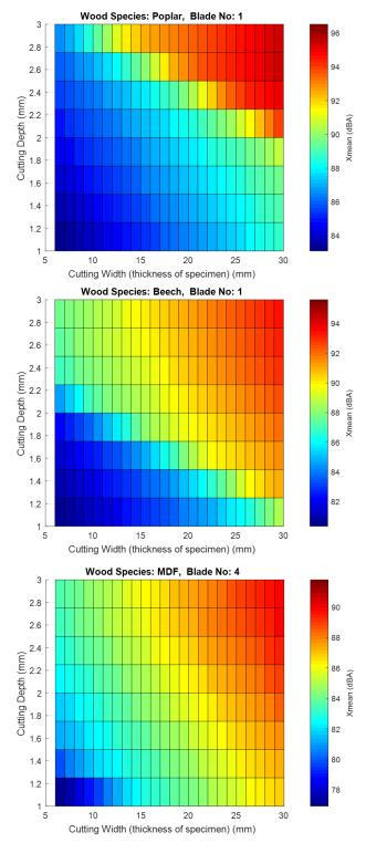
FIGURE 4: Predictive changes in noise emission for different cutting widths and cutting depths.
