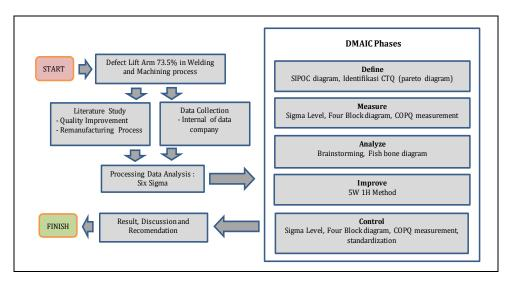
Figure 1. Research Methodology of Problem Solving Lift Arm in Welding and Machining Process
