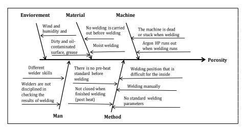
Figure 5. Cause and Effect diagram of product failure Porosity
