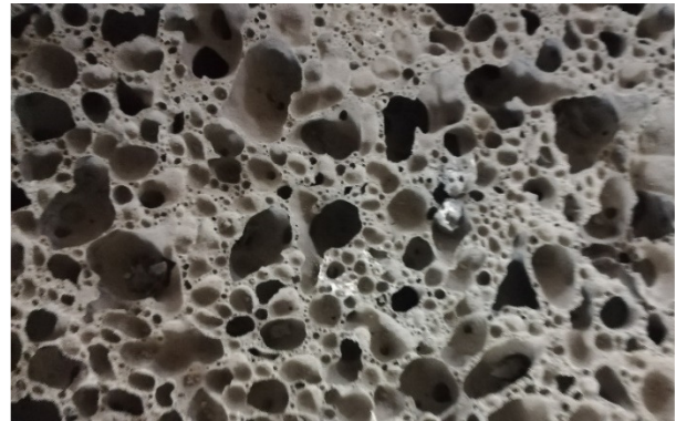
(b) Fly-ash-based geopolymer fed using hydrogen peroxide
