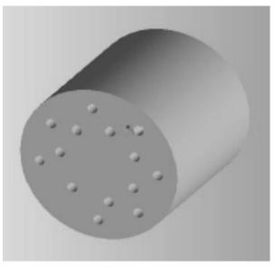
Figure 2. Cylindrical coal briquettes designed for this study.
