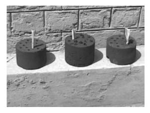
Figure 6. Cylindrical coal briquettes drying in the sunlight.
