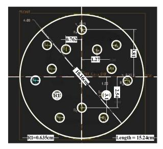
Figure 3. Mechanical layout of the coal briquetting cylinder.
