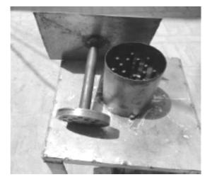
*Figure 5.* Top view of the compression cylinder with top circular steel plate with holes to slide inside the cylinder under the influence of sufficient load.
