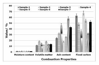
*Figure 7.* Measured combustion properties of samples used in this study (sample numbers correspond to the compositions given in Table 2.
