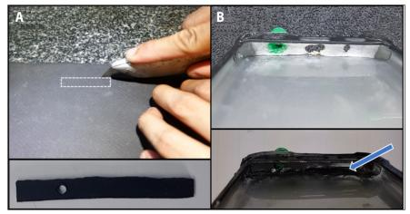
Figure 2 A. Using a craft cutter, a 70mm x 5mm x 2mm EVA rubber sheet was taken from a mouse pad; B. Sound-proofing; arrow points to EVA rubber sheet glued to inner bottom compartment of case.
