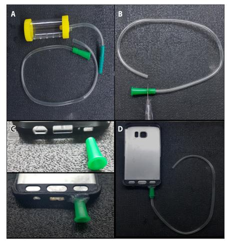
Figure 1 A. Simplex\* Mucus Extractor, detached suction attachment and PVC tubing; B. Cutting suction attachment (Sound port) from tubing (Intra-oral attachment); C. Attaching sound port using cyanoacrylate glue; D. Phonetovox (360 full shell casing with soundport and intra-oral attachment).
