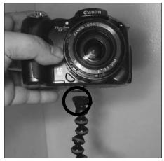
Figure 7b. Camera with attached quick release plate (circle)
