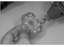
Figure 2a. 12-LED bulb headlight with adjustable mount
