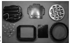
Figure 2 b. Components of disassembled headlight
