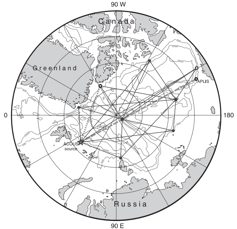
Fig. 2. A notional monitoring grid for the Arctic Ocean. The stars represent the three autonomous acoustic sources. The filled and open circles indicate the cabled receive arrays and Arctic Ocean observatories. The open circle in the Lincoln Sea represents an existing sea–shore interface. The open circle in the Beaufort Sea represents a sea–shore interface which does not yet exist. The open circle in the Chukchi Sea shows the APLIS Ice Camp location. The short-dashed grey line from the ACOUS source to the Lincoln Sea is the acoustic path along which acoustic thermometry transmissions were made from October 1998 to December 1999. The long-dashed grey line is the acoustic path from the ACOUS source to the APLIS Ice Camp in the Chukchi Sea along which acoustic thermometry measurements were made in April 1999.
