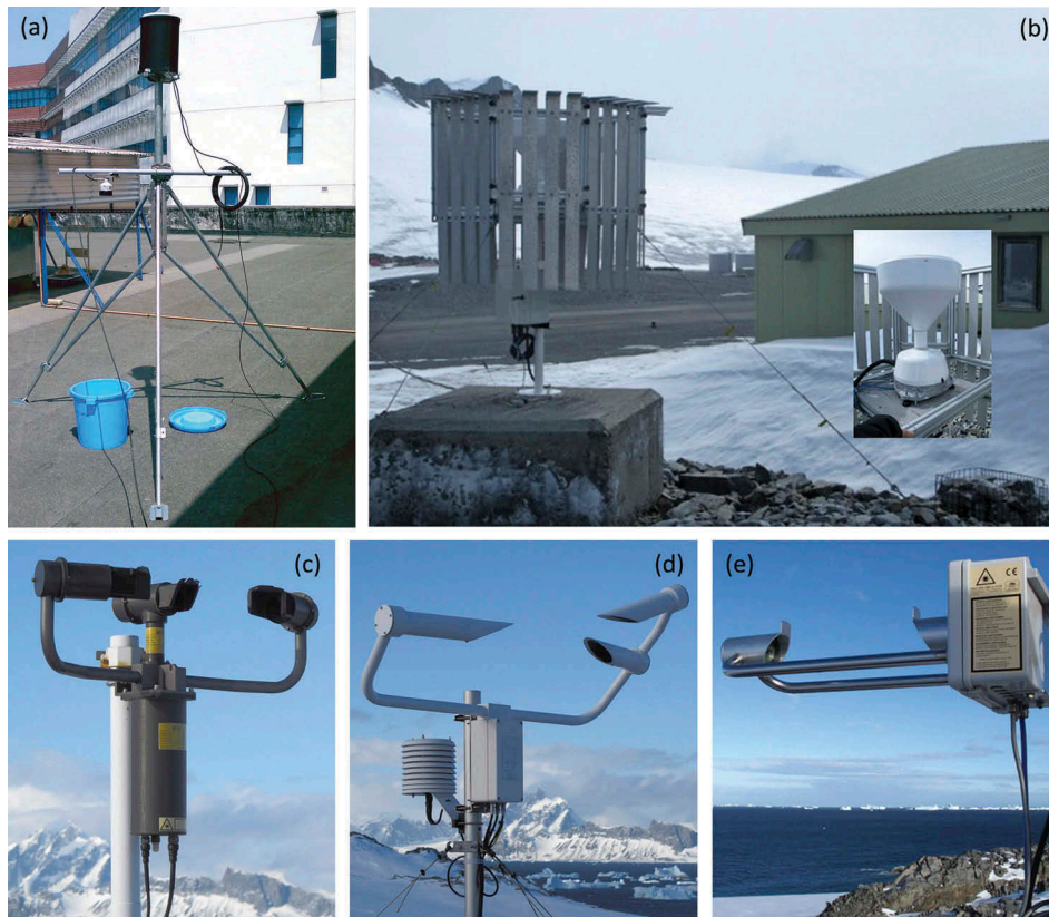
Figure 1. (a) The CS700H, seen here with the SR50 snow depth sensor (on the left on the horizontal rod), undergoes a test at a site at the University of Malaya before deployed to Rothera. (b) The wind shield installed around the UPG-1000 (inset). (c) A VPF-730 sensor. (d) PWS-100 installed at Rothera Station. (e) An LPM installed at Rothera.
