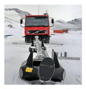
Crevasse-detecting radar developed by the Norwegian Polar Institute. Mounted in a 12-m forward boom in front of the lead vehicle, the device allows the driver to monitor the structure of the ice down to 30 m below the surface, and thereby to avoid crevasses. (Photo by Jan-Gunnar Winther; courtesy of Norwegian Polar Institute Photo Library.)
