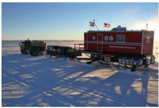
The four tracked vehicles each pulled two sleds loaded with fuel, equipment, and living and working quarters. (Top photo by Atsuhiro Muto. Bottom photo by Stein Tronstad; courtesy of Norwegian Polar Institute Photo Library.)
