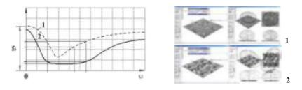
Fig. 1 – The dependence of the coefficient of sliding friction  $f_0$  from speed v for planar contact:
