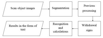
Fig. 4 – Generalized scheme of the process of optical recognition of objects
