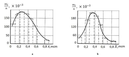
Fig. 5 – Histograms of the distribution of superhard grains on the working surfaces of the cutting plates by the numbers of grains: a - 14/10; b - 10/7
