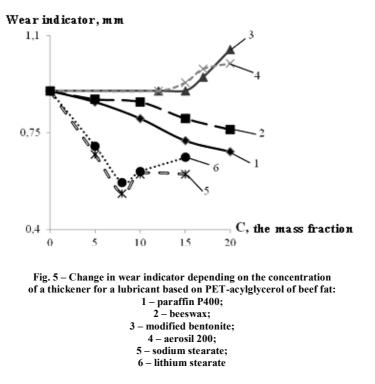
Paraffin and beeswax somewhat reduce the wear indicator at a concentration of 10 m.f. to 20 m.f., at low content their presence in no way affects the process of wear of the material. The low content (from 12 m.f. to 15 m.f.) of inorganic thickeners did not affect the change in wear indicator, however, with a further increase in concentration (from 17 m.f. to 20 m.f.) there is an increase.
